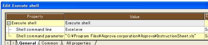
▲ Fig. 4 Command line and argument assigned to the Execute shell command
